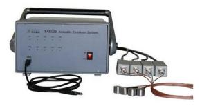
Figure 11. SAEU2S Acoustic Emission Instrument
