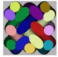
Figure 2. three-dimensional(3D) and four-directional(4Dir) braided architecture
