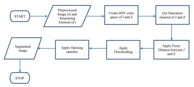
Figure 2. The Step Process of Image Segmentation Phase of the Proposed Method
