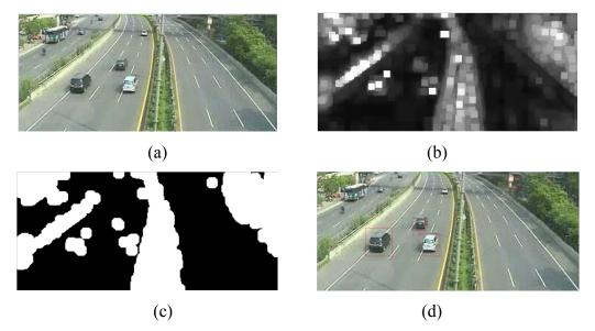
Figure 5. The Experimental Result of Each Phase of the Proposed Method: (a) Original Image (b) After Fuzzy Dilation Process (c) Segmented Image and (d) The Result of Vehicle Detection By manual counting, the accuracy rate can be quantifiably calculated. Here, the result of counting vehicles manually is considered to be the correct result, as presented in Table 1.
