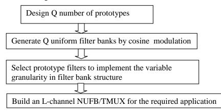
Figure 3 Flow chart for variable granularity bands using multiple prototype filters
