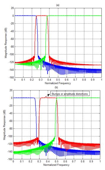
Figure 7 Variable granularity bands from multiple prototypes (a) Example 1: Proper combiners (b) Example 2 : Improper combiners with amplitude distortion
