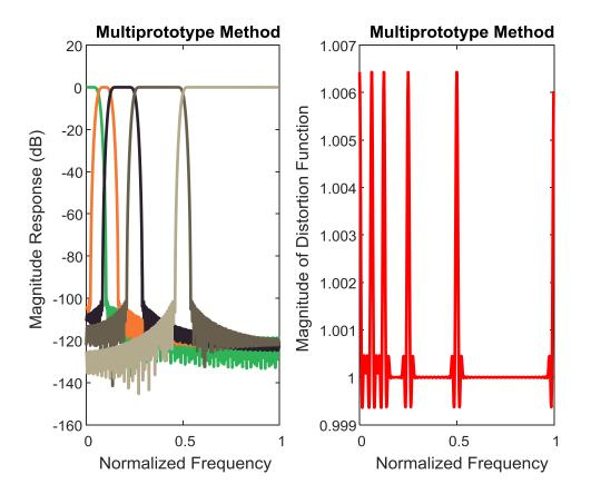
Figure 4 Non uniform Filter bank design using *single and multiple prototype methods* and the corresponding distortion functions
