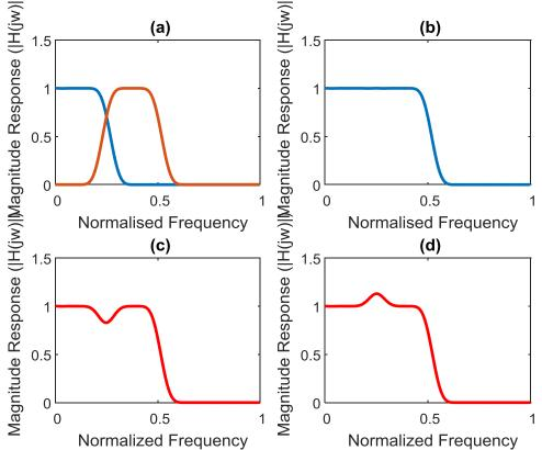
Figure 2 Frequency Response when adjacent subbands are combined (a) Adjacent uniform subbands (b) Addition of subbands at 3dB (c) and (d) Addition at points before and after 3dB creates distortions in the form of dips and bumps.
