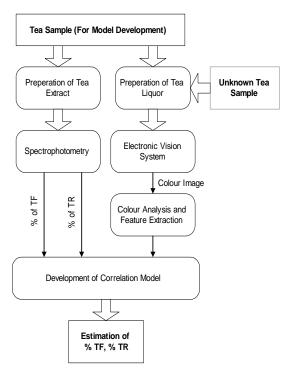
Fig. 1. Operational Flow chart of the overall experiment
