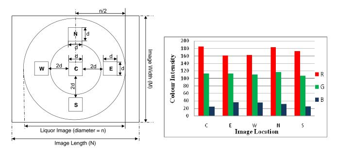
Fig. 4. Captured image with marking of different regions (C, N, W, S, E) from where colour based different image features were extracted.
