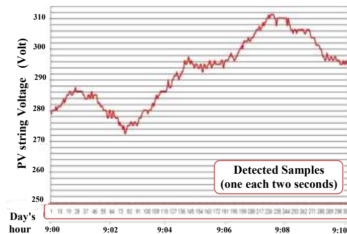
Figure 27 Plot, as function of time, relative to DC voltage samples acquired from PV string during a short time interval of the morning.
