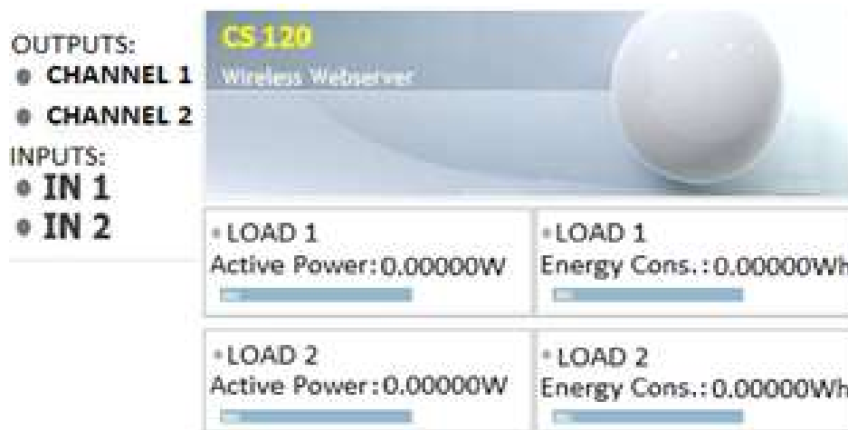
Figure 21 Screenshot of realized web page in order to switch on/off the connected electrical loads and view, after current data processing, instantaneous active power (W) and overall consumed energy (Wh).
