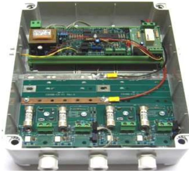
Figure 32 Photo of designed and realized control panel of PV plants including the circuitual sections of parallel connection, strings protection, detection and processing of PV plant parameters and alarm anti-theft.
