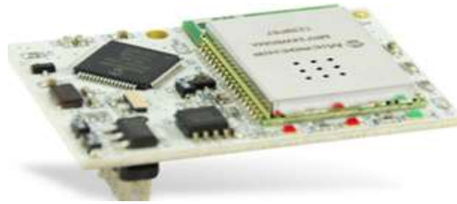
Figure 18 Open Picus FlyPort board with embedded the WiFi module.
