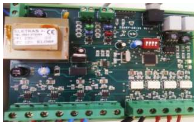
Figure 24 Photo of the CS097 realized electronic board, for acquisition / processing of PV plant data, after the mounting of SMT and through hole components.
