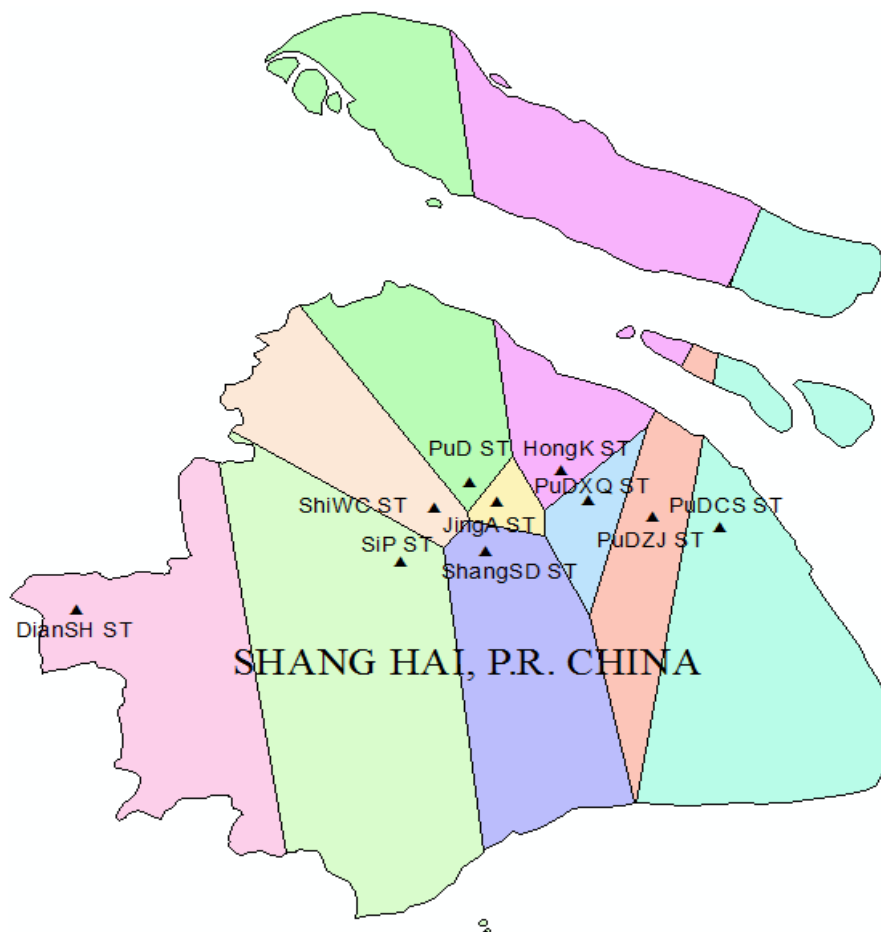
Figure 7. Generated Thiessen polygons and the monitoring site location
