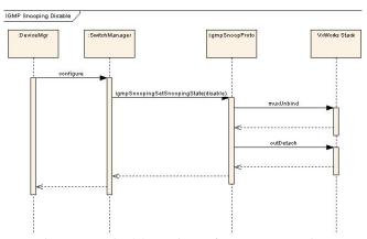
Figure 8. Disable action of IGMP snooping
