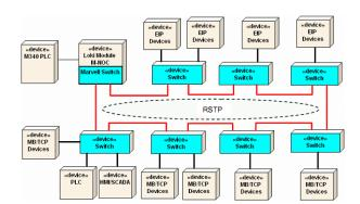
Figure 4. The switch ring network topology with the C1 module
