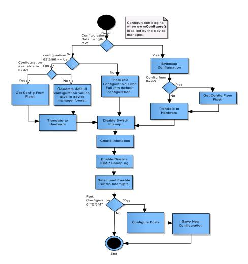
Figure 6. Switch manager configuration flow chart
