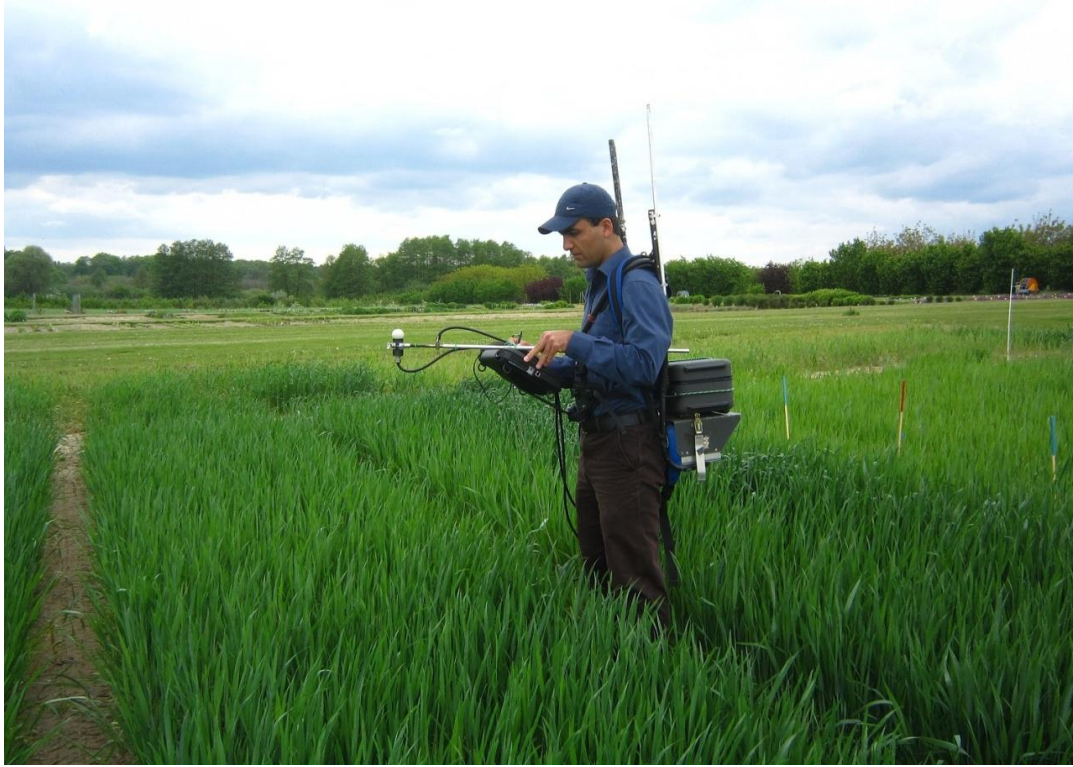
Figure 3. The spectroradiometer used for spectral spot measurements
