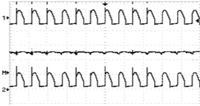
Figure 13. Typical Unipolar Control of PMBLDC motor using Hall sensor and IGBT-without current chopping
