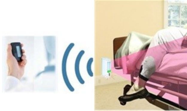
Figure 12. Wireless signaling between PIR motion sensor and the caregiver pager
