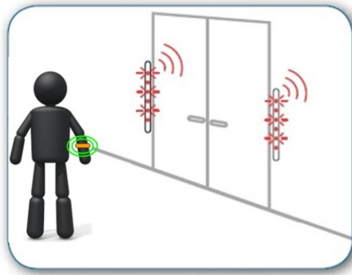
Figure 10. An example of the anti-wandering wristband based door alarm system
