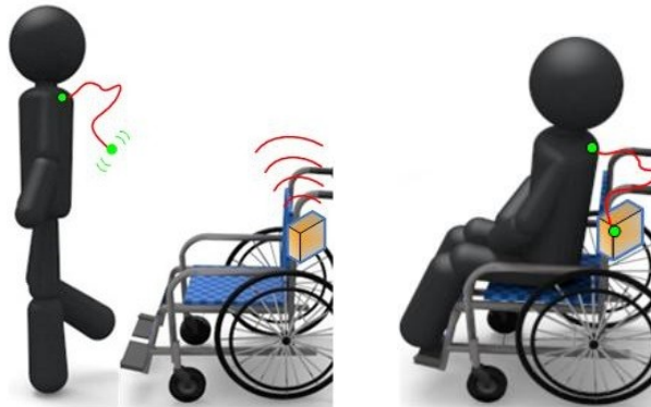
Figure 8. An example of wheelchair pull-string monitor
