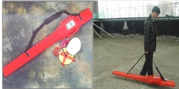
Fig 2: Multi-frequency electromagnetic profile-measuring instrument (GEM300)
