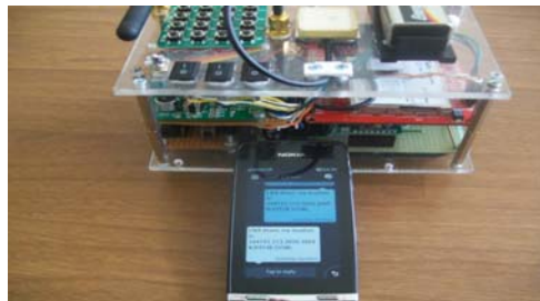
Figure 9: Testing GSM-GPS Module and Accelerometer Sensor.
