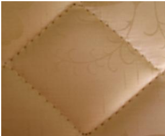
Figure 13. Quilting effect of 4.5mm thickness workpiece
