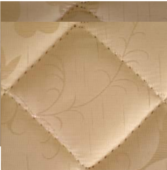
Figure 13. Quilting effect of 4.5mm thickness workpiece
