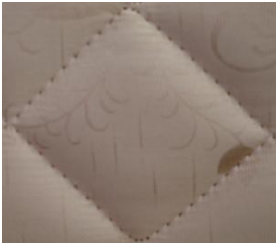
Figure 12. Quilting effect of 5.5mm thickness workpiece
