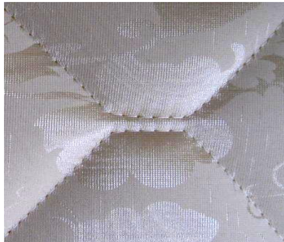
(b) No deformation of the angle of two lines after compensation (Bending corner)
