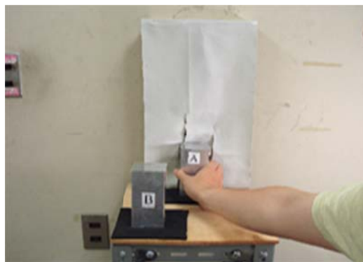
Figure.10 Experimental method for lifting a PAO. The human lifts the PAO (A) and compares its weight to that of the MLO (B). The main PARS is hidden behind the PAO in order to eliminate any visual differences between the MLO and the PAO.
