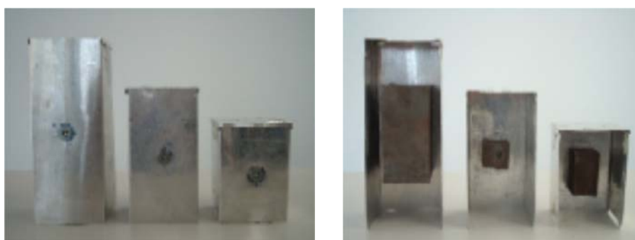
Figure. 2 Fronts and backs of different sizes of MLOs. The left photo, from left to right, shows the front sides of the large, medium and small MLOs respectively. The right photo, from left to right, shows their backs. The extra mass attached to the back of each object is also shown as examples. Extra mass helps change the weight keeping the front view unchanged.
