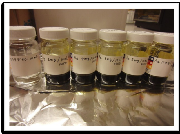
Figure 3. Silver nanoparticle ink adjusted for LIBS measurement
