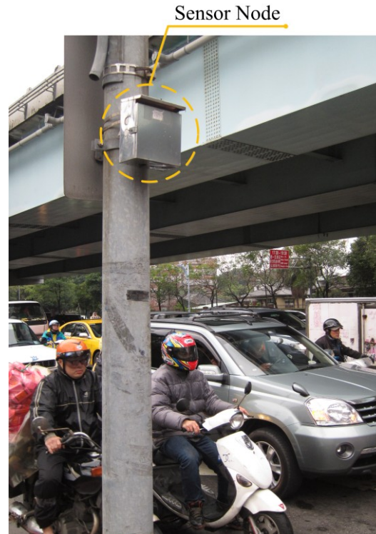
Figure 19. Deployment of the air quality monitoring system. A sensor node was attached to the traffic signal pole
