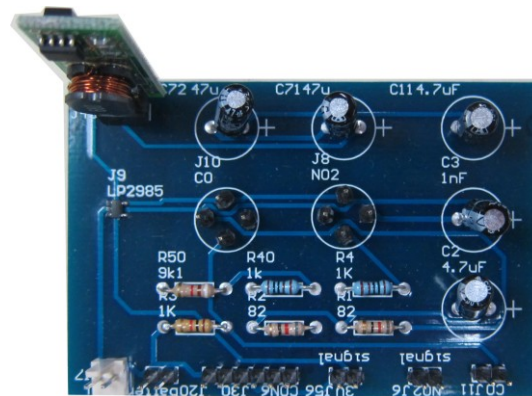
Figure 8. The sensing signal processing module
