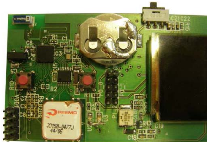
Figure 4. Tag is the same size as a normal credit card (8 cm x 4 cm). It consists of a CC2430 SoC, AS3931 LF-receiver, two buttons, and an OLED-display.
