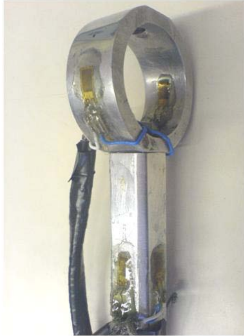
Figure 7. The 3D force sensor realization
