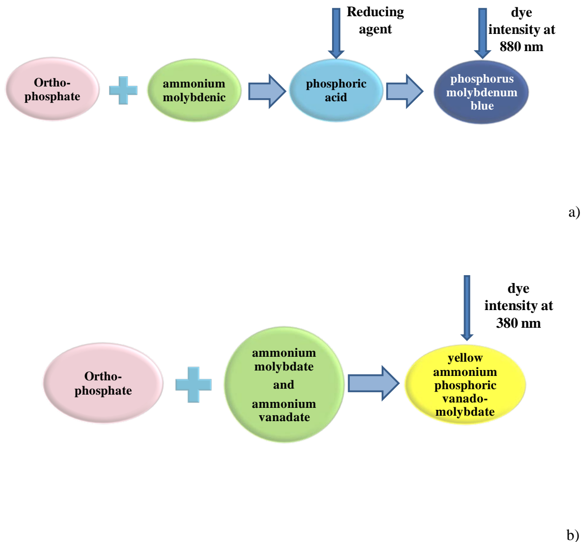
Figure 2. Conceptual diagram of standard UV-Vis optical methods: a) Molybdenum blue method, b) Vanadate / molydate yellow method.
