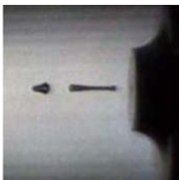
Figure 9. Bursting of ink-drop at a high voltage over 3.5kV.
