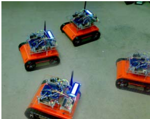
Figure 14. Al-Fath – Robot for odor source localization
