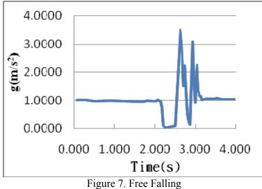
As shown in the figure, at about 2.5 sec, a small interval of zero gravity state lasts for a while. Afterwards, there is an acceleration surge, indicating impact after free fall. Therefore, the algorithm is defined as below, where time T depends on danger altitude:
