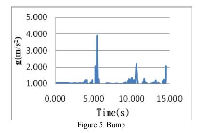
Therefore, the impact algorithm should include monitoring of number and time of occurrence, where C is at critical value marked Stable in Table 1, e.g.,  $N_{Gstable}$  denotes acceleration when neck is stable, and T denotes system preset time. Hence, the algorithm can be defined as follows:
