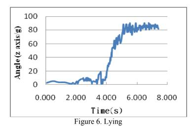
In this system, the upper body angle can be calculated based on waist and neck acceleration data. When it is observed that body angle increases suddenly, and is under impact, it can be inferred that the user encountered an accident. Later data will record the impacted position of the fall, and accident incident will be documented. System algorithm is expressed as follows, where C is critical angle of lying, or  $W_{ANGstable}$  and  $N_{ANGstable}$ , as shown in Table 1:
