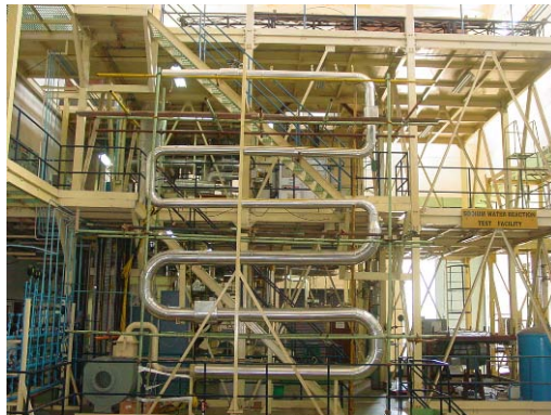
Fig. 1. Test loop to test optical fiber based distributed sensor for temperature sensor
