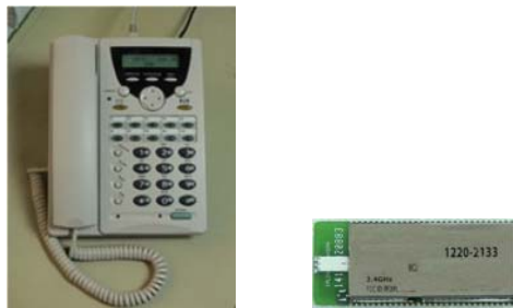
Fig. 6. LRPWAN device (right photo), a lighter size module, is used as a tag in user's pocket, or as a sensor node on IP phone (left photo).
