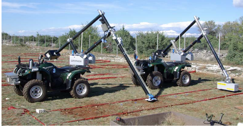
Figure 9: Gryphon dual-sensor system, composed by metal detector and GPR (left) MD-Gryphon, (right) GPR-Gryphon
