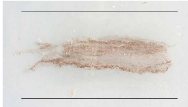
Figure 8. Photo of the burn-in pattern as a result of PTI testing at a voltage of 400 V using horizontal chisel-shaped electrodes; Distance between the electrodes (black lines) is 4 mm.
