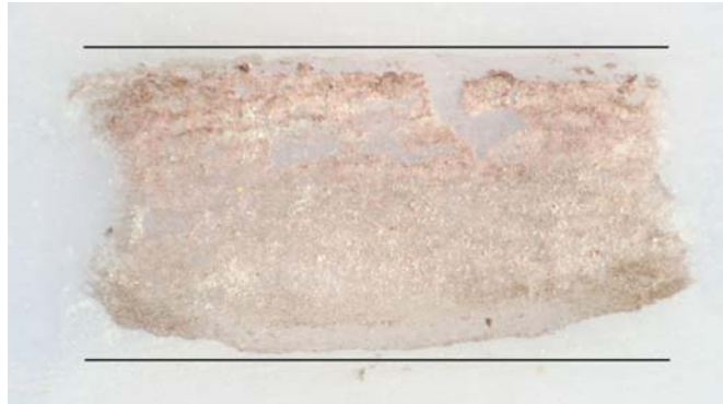
Figure 11. Photo of the burn-in pattern as a result of PTI testing at a voltage of 400 V using thin horizontal electrodes; Distance between the electrodes (black lines) is 4 mm.
