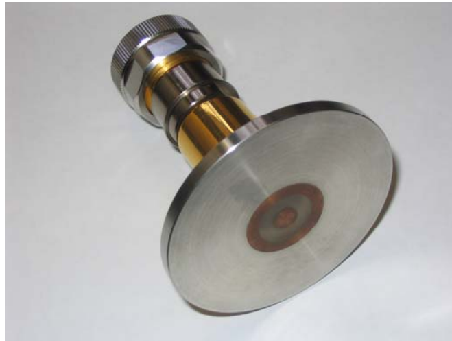
Figure 1. Coaxial probe fabricated from air line.
