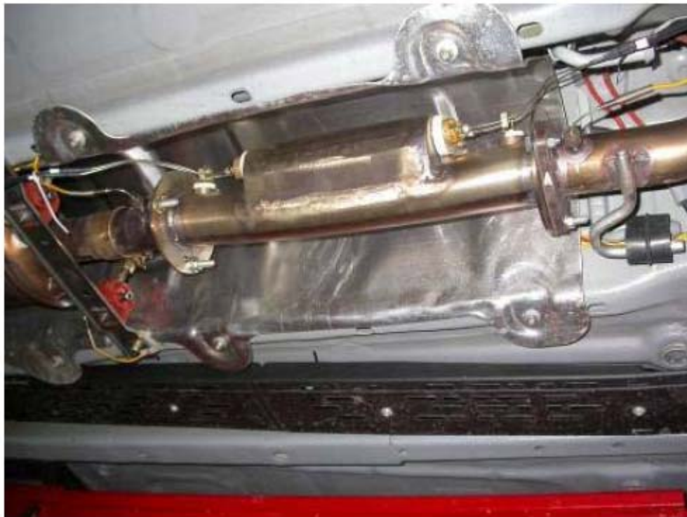
Figure 8 The UV Gas Sensor Mounted Underneath the Car
