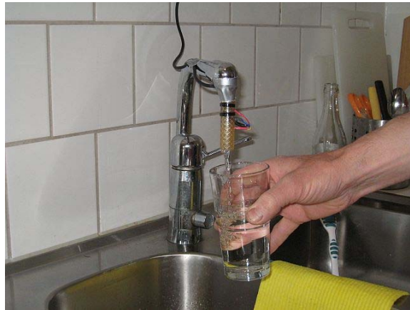
Figure 5. The electronic tongue device on the water tap
