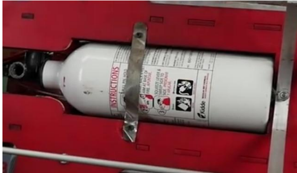
Figure [5] – attaching fire extinguisher tank to the quadcopter base
