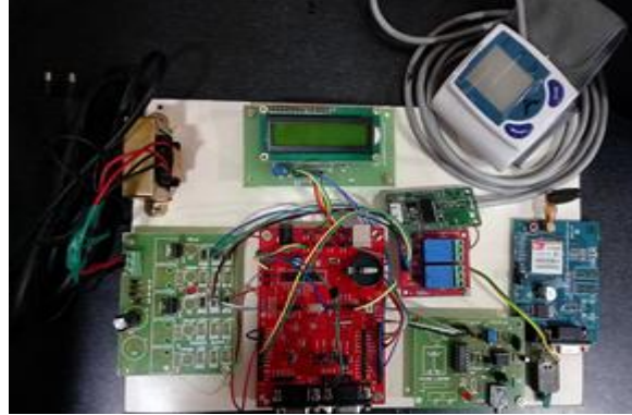
Figure.11 Interfacing of BP sensor and GPRS module
