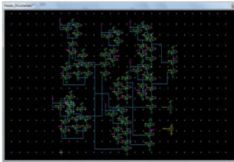
FIGURE 6.5.SVL MODIFIED CMOS CURRENT COMPARATOR WITH PSEUDO NMOS LOGIC
