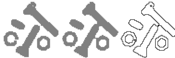
d) Opening with 2B e) Closing with 2B f) Hit-and-Miss with B_1 and B_2
