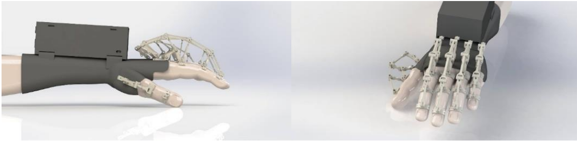
Figure 5. CAD model: flexion state
