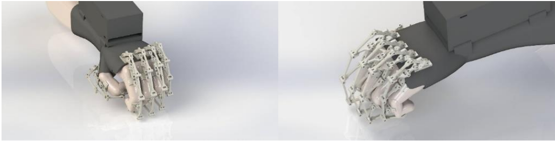
Figure 4. CAD model: spring-return flexion mechanism (rest state)
