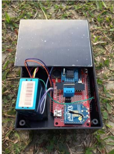
Figure 10. Set up XBee module on WEMS
