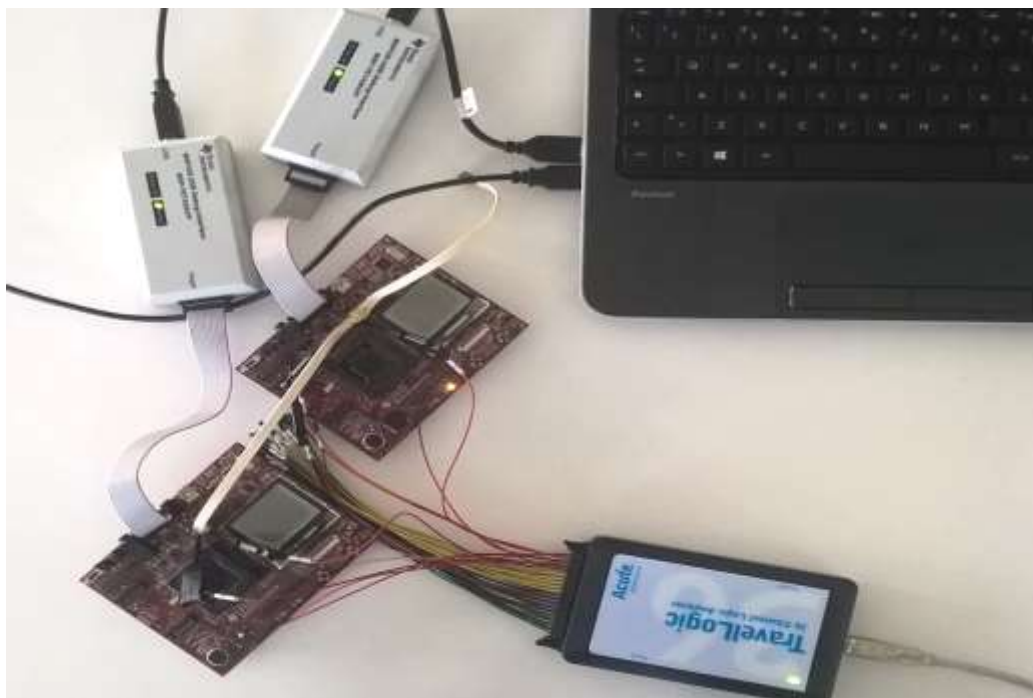
Figure 22. Realized experimental setup for SPI communication.
