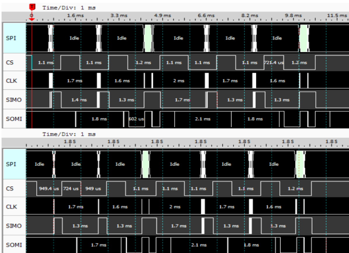
Figure 44. Detail of the two ping procedure performed before and after that the first slave negotiated a new speed.
