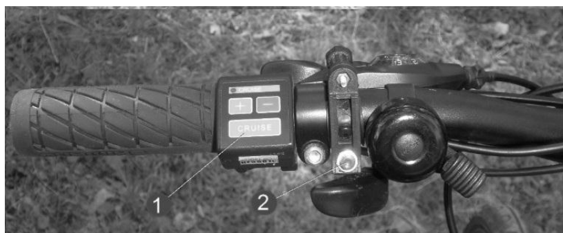
Fig. 4. Operating elements on the left handle: 1 – cruise control; 2 – the button for regenerative stopping
