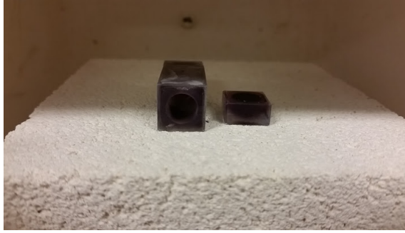
Figure 4.8: A Eu:CaF 2 vapor cell after exposure to calcium vapor in vacuum at 650 °C, observe the purple color of the cell, no longer transparent to either the 423 nm cooling or the 657.3 nm clock transition.
