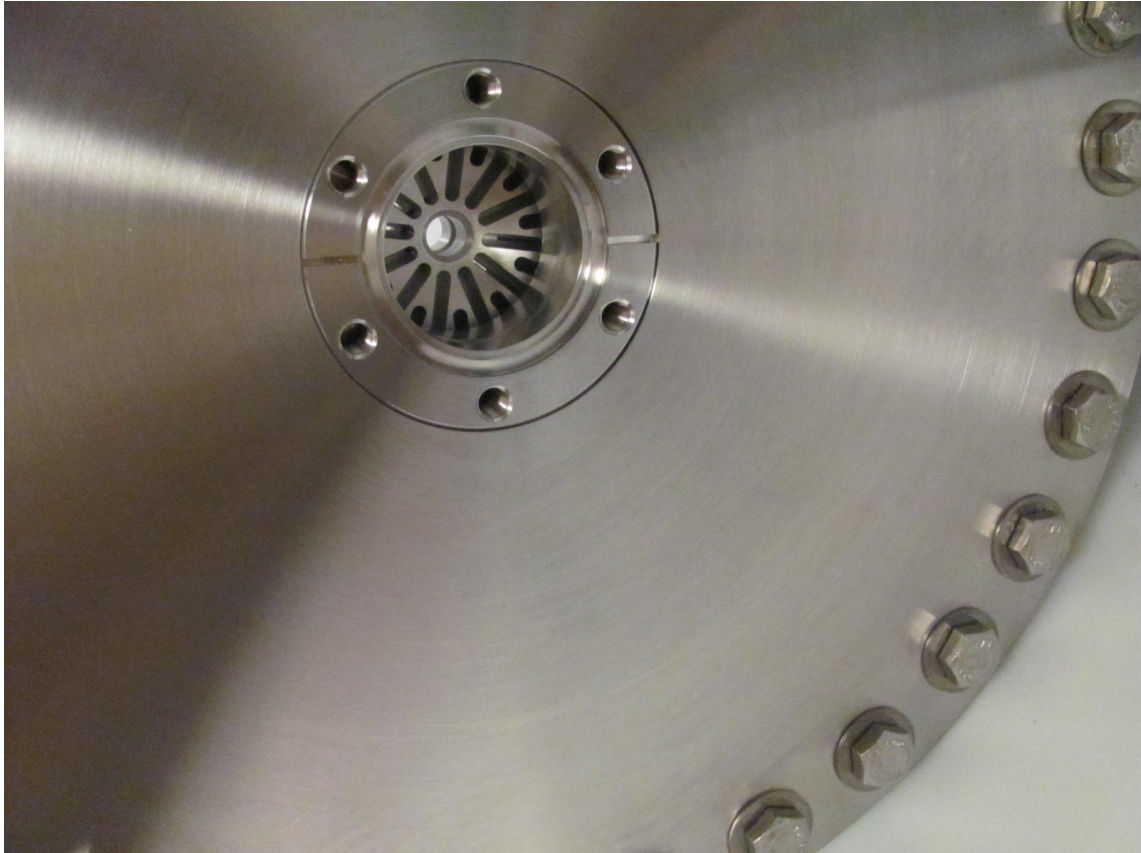
Figure 1.1.6: The cavity of Figure 1.1.5 sandwiched between two 12" to 2¾" flange reducers to make it compatible with Jlab's Injector Test Facility beamline.
