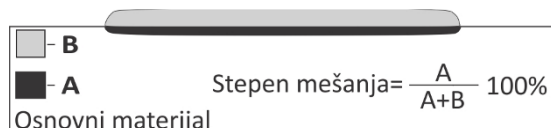
Slika 2. Način izračunavanja stepena mešanja OM i DM Figure 2. Method of calculating dilution of the base material and the filler material
