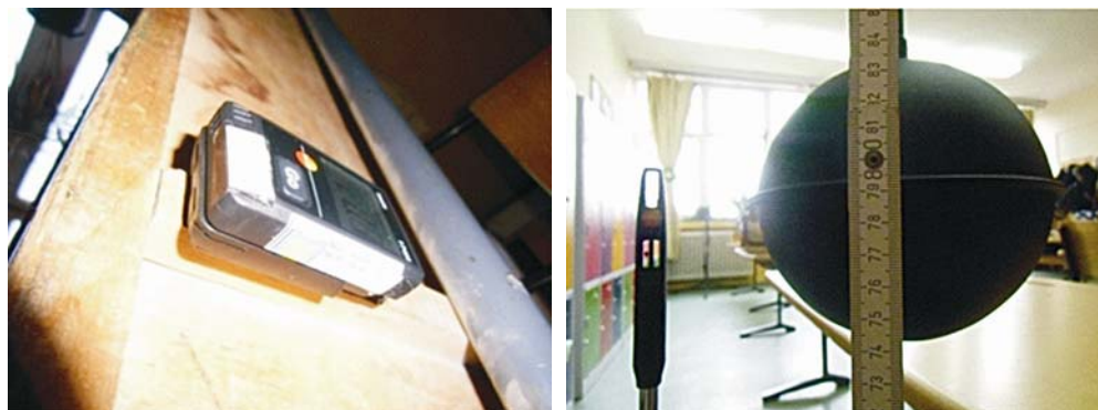
Figure 3. Thermal comfort data loggers, black globe, and hot-wire anemometer
