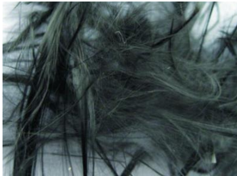
Fig. 2.3. Low bulk density (fluffy), randomly oriented dry fibre format of rCF from pyrolysis 139 .
