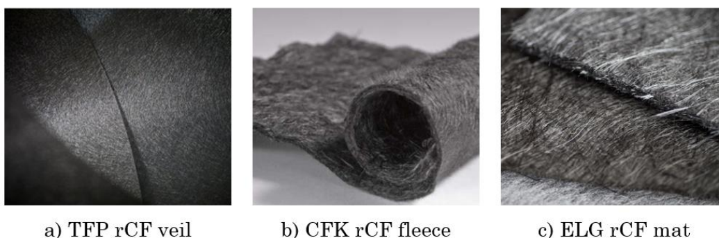
Fig. 2.4. A range of commercially available rCF nonwovens of varying areal weights 65,67,146 .
