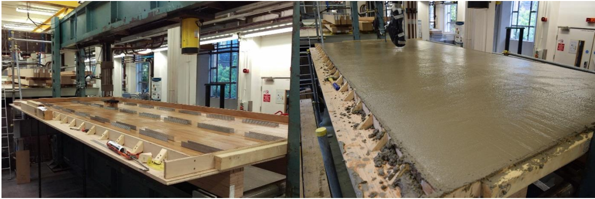
Figure 6 - Formwork for three-joint specimen (a) before concrete pour, and (b) following the concrete pour
