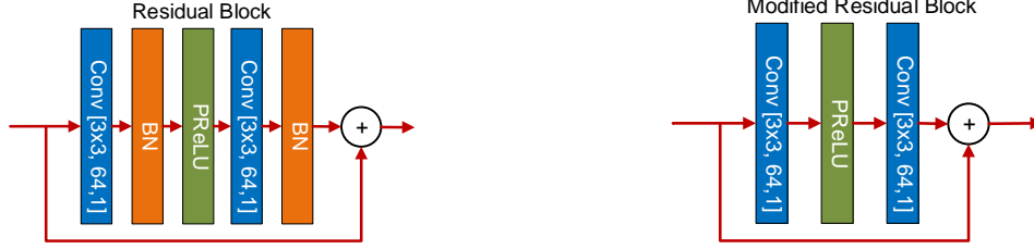
Figure 3. (Left) The original residual block in SRGAN. 10 (Right) The modified residual block in M-SRGAN
