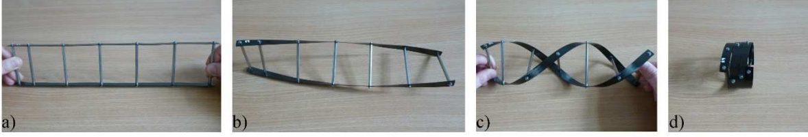
Figure 2: Manufactured prototype of the double-helix structure in a) straight, b) stable twisted, c) unstable twisted and d) fully coiled configuration.
