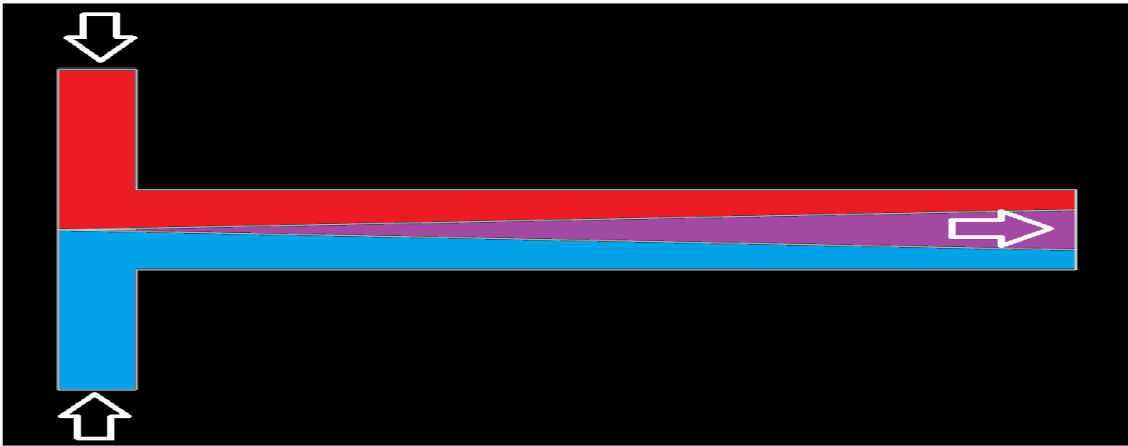
Figure 4: Simplified T-mixer design. Red and blue shows the two unmixed streams and purple shows the completed mixed stream. The mixing increases as time progresses.
