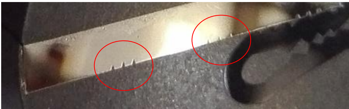
Figure 42: Zoomed in section of figure 42 showing penetration depth of the ablation.
