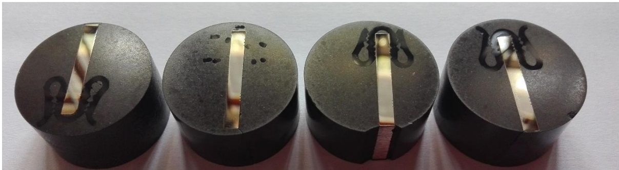
Figure 41: Cross-sectional cuts of Hastelloy plates that is polished in a conductive resin inlay.
