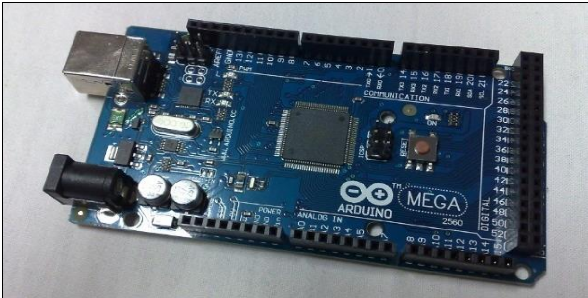
Figure 30: Clone of an Arduino Mega Development board (Dragan Simic CC4.0)
