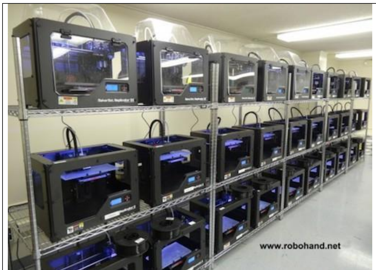
Figure 14: FDM 3D printing farm (Public Domain)
