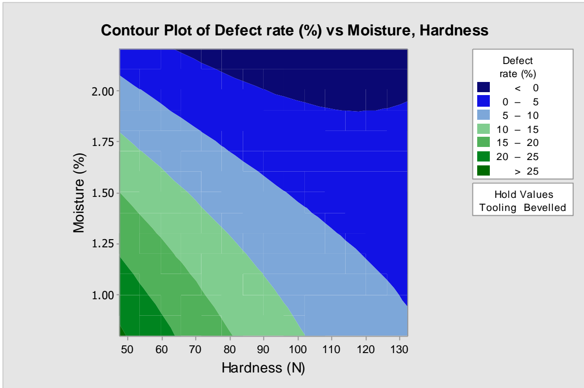
Figure 4.3: Bevelled tooling - Contour plot of Defect rate (%) vs moisture, hardness.
