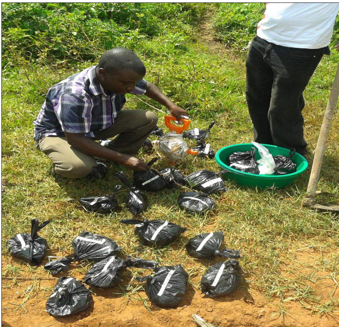
Figure 3.4: Collection and labeling of soil samples in preparation for laboratory C analysis
