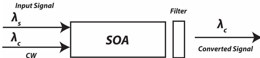
Figure 5.9: SOA cross gain modulation wavelength converter (Ramamurthy & Mukherjee, 1998, p. 1061- 1073).
