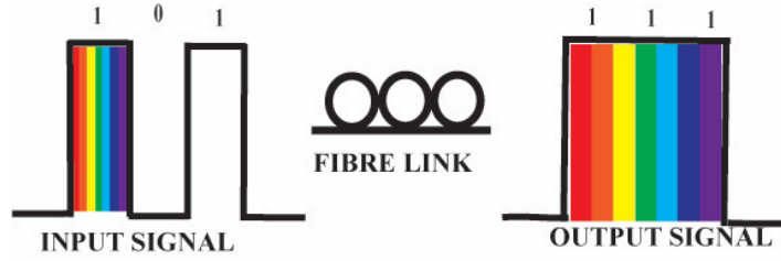
Figure 5.5: Chromatic dispersion effects in an optical fibre.
